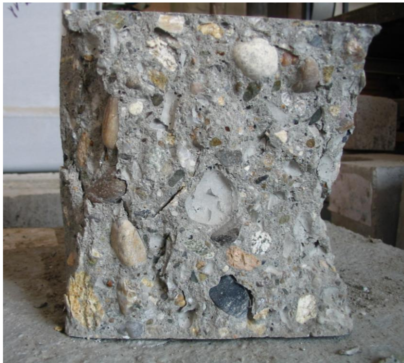
Fig. 5. Way of fracture of cubic concrete sample under centric compressive stresses with friction on the contact faces
