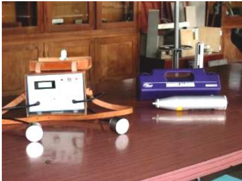
Fig. 5 Ultrasonic apparatus and test hammer
