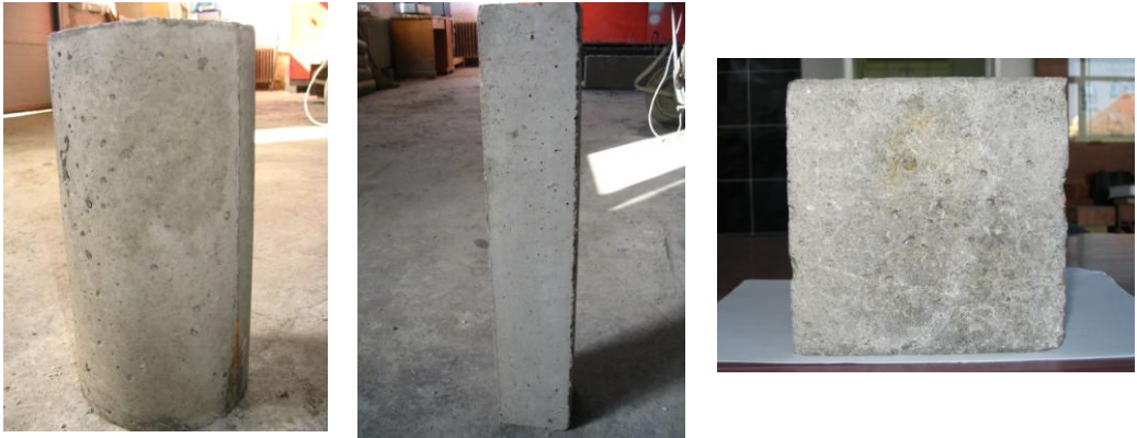
Fig. 6 Cylindrical, prismatic and cubic concrete samples
