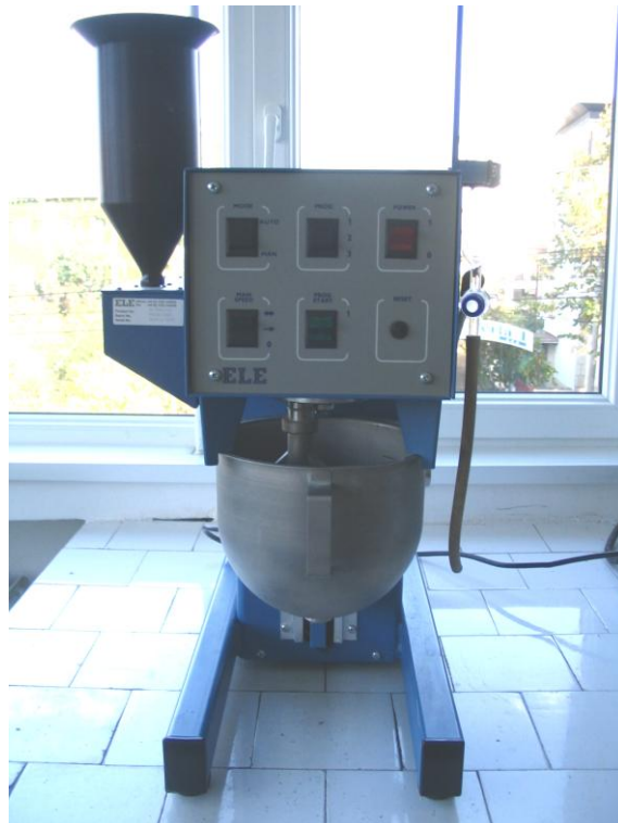
Fig.6 The mixing machine for preparing the mortars
